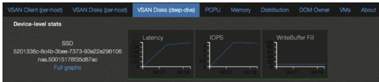
Figure 5.19 - vSAN observer write buffer fill info
